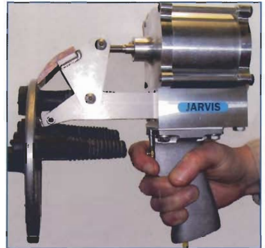
Jarvis' PFC-1 Picking Finger Cutter doing its job.
